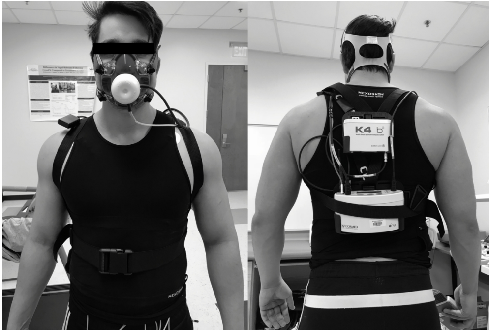
Configuration of Cosmed (K4b2) device for each participant
