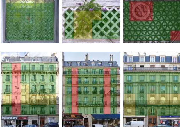
Figure 5. Examples of ground truth image annotations. We define a regular grid and label each cell as green (instance of a repetitive item), yellow (instances with strong appearance changes) or red (not an instance of the repetitive pattern).
