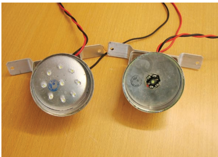
Fig. 5. White LED luminaires manufactured in Nepal for rural village lighting using Nichia NSPW510BS LED (left) and Lumiled's Luxeon Star LED (right).
