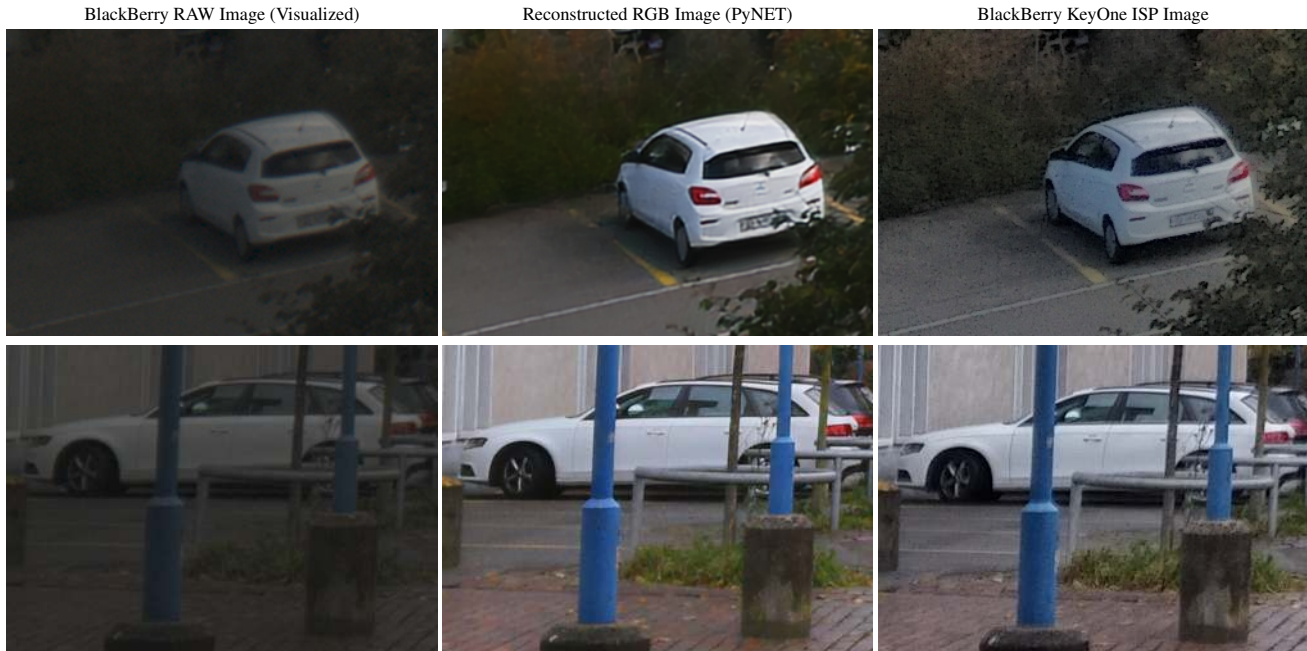
Figure 8. Image crops from the BlackBerry KeyOne RAW, reconstructed and ISP images, respectively.
