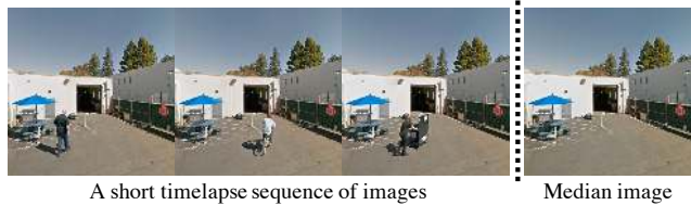
Figure 2. Our dataset consists of short image bursts, i.e. , short timelapse sequences of images captured over several seconds. We compute the median of each timelapse image stack to produce a “clean plate” background image free of objects and shadows.
