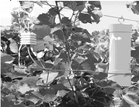
Fig. 1. PVC container for Mote hanging in a vineyard with Stephenson screen
