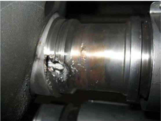
Figure 16: Damage due to secondary arcs in QQBI.27R3 (left) and QBBI.B31R3 (right)
