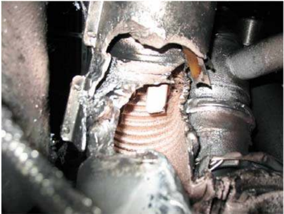
Figure 16: Damage due to secondary arcs in QQBI.27R3 (left) and QBBI.B31R3 (right)
