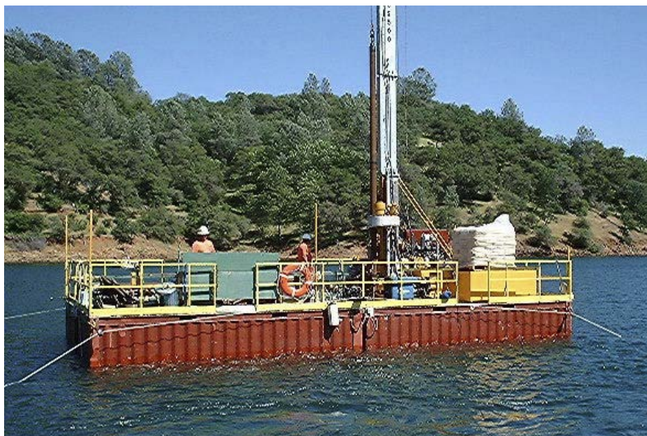
Figure 2. Photograph of the GLAD200 coring rig on Englebright Lake.
