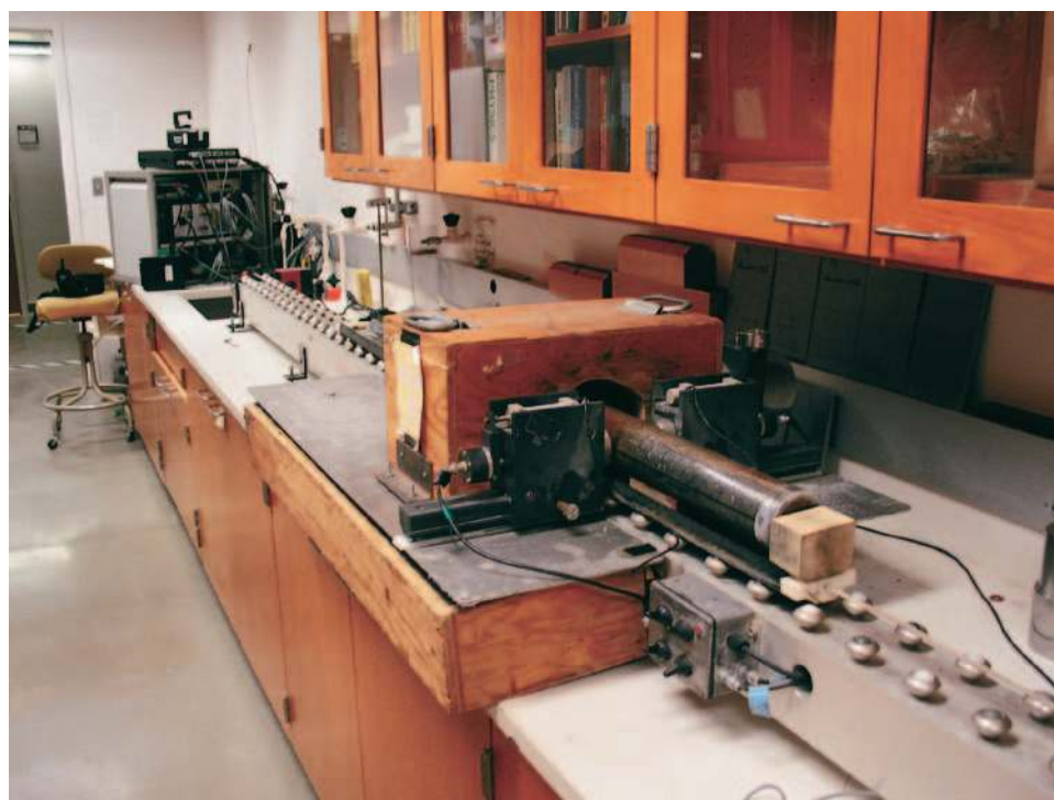
Figure 5. Photograph of the multisensor core logger used in this study.
