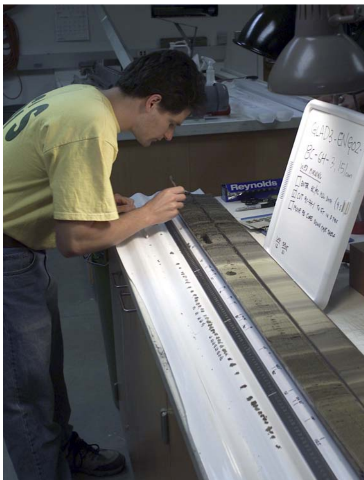
Figure 6. Photograph of core visual descriptions.
