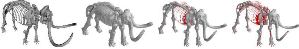
Figure 5: As-manufactured models shown for a small cylindrical feature F with a shape S representing the skeleton of a woolly mammoth [1]. Reading clockwise from left, the nominal model is shown first. Subsequent images show \lambda = \frac{\epsilon}{\mu(F)} , \lambda = \frac{1}{4} , \lambda = \frac{3}{4} respectively. The as-manufactured models are shown in silver and the unincluded regions of the original part are shown in red. When \lambda = 1 (bottom left) F is constrained to remain within S and the regions visible in red indicate regions of S where F cannot fit. For \lambda = \frac{1}{4}, \frac{3}{4} it is seen that the as-manufactured model contains significant areas where material is deposited outside the original part boundary. \lambda = \frac{\epsilon}{\mu(F)} represents the Minkowski sum of F and S . Indicator functions of input solid models are sampled on a grid size of 256^3 to compute the convolution.
