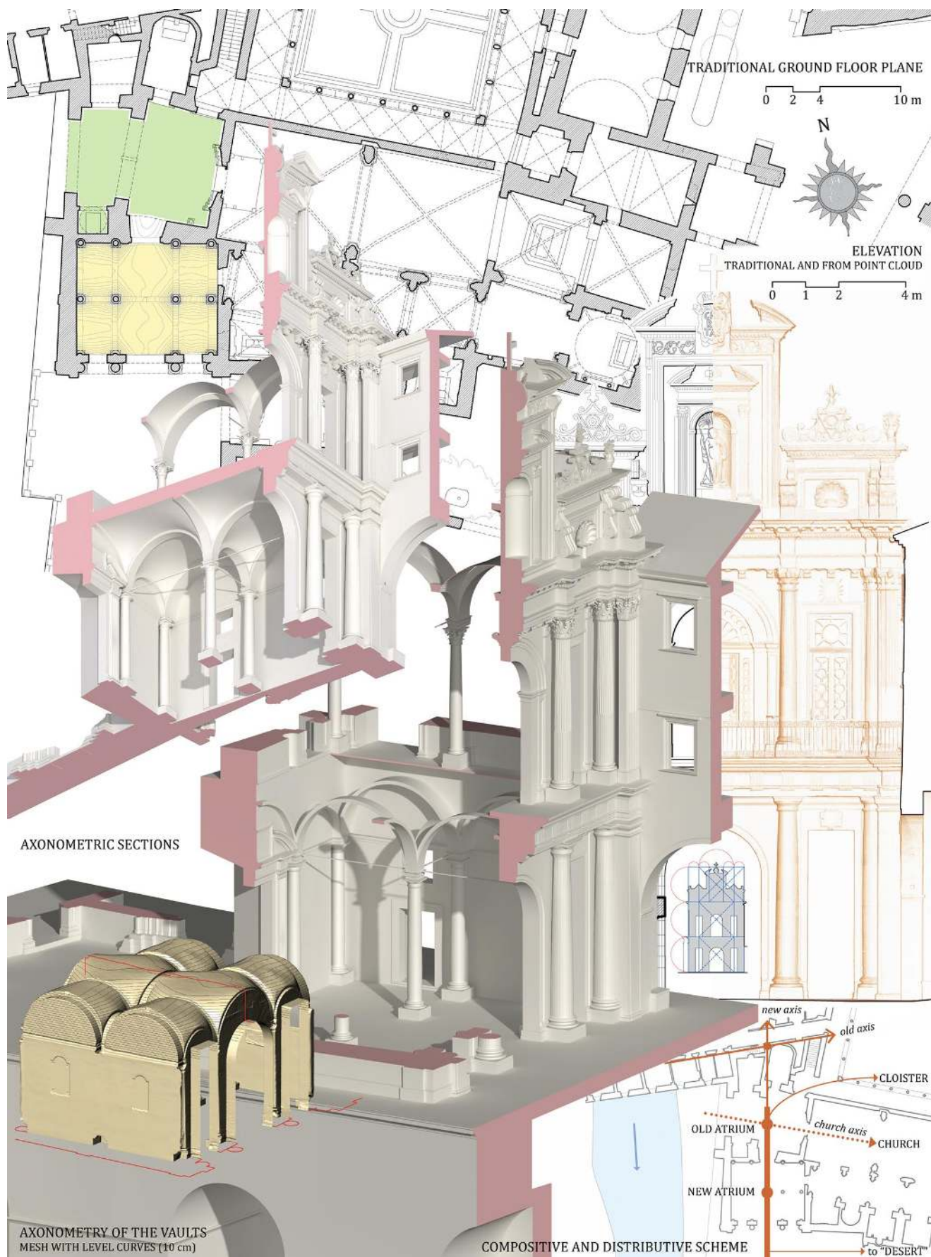
Fig. 6: Survey of the atrium of the convent of St. Francis of Paola; figurative device constructed by a simplified 3D model and consisting of drawings dedicated to the architectural theme of the atrium and to the geometries of the vaults on the ground floor.
