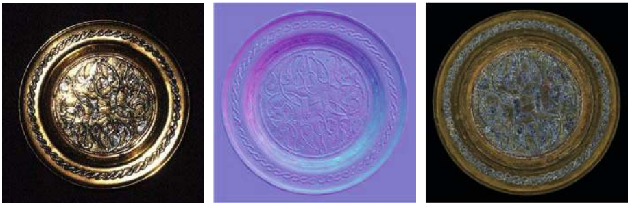
Fig. 12. Damascene dish: (left) image illuminated by four lamps in tier 5 of dome; (centre) normal vectors in false colour; (right) albedo
