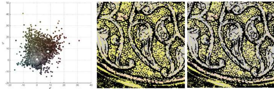
Fig. 17. (left) 10,000 pixels plotted on the CIELAB a^*-b^* chromatic plane, with centroids for the three metals; (centre) classification by hue angle; (right) classification by nearest colour
