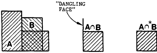
FIGURE 3. The regularized intersection of two r -sets is an r -set, but their conventional intersection need not be regular (sets shown in orthographic projection).
