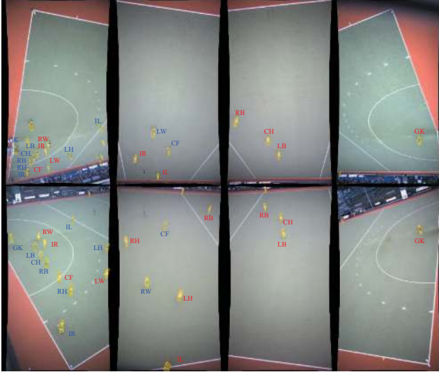
Figure 7. Players are detected by interpreting background subtraction results in terms of 3D geometry, where players are coarsely modeled as cylinders. Based on these detections, we assign player role for each team.
