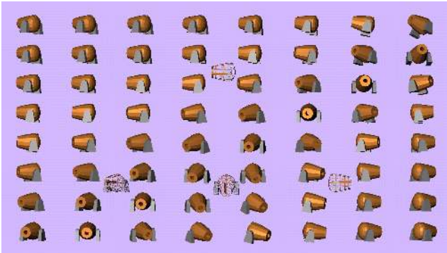
Figure 7: The affine combination of orientations. Each orientation on the grid is computed as an affine combination of four key orientations depicted as wireframes. Weight values are determined to provide a smooth parameterization on the xy plane using radial basis functions.
