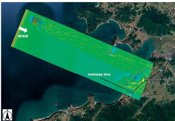
FIGURE 7: Wind speed distribution in the mainstream direction x , instantaneous flow field, and horizontal cross-section 5 m above ground.
