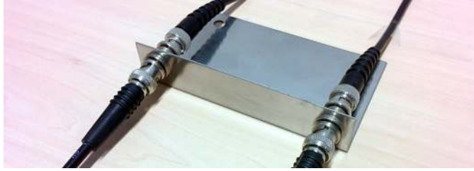
Figure 8.10: RG-58 and BNC feed-throughs without a ground plane.
