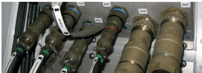
Figure 8.1: EMC connectors with 360° EMI backshells.
