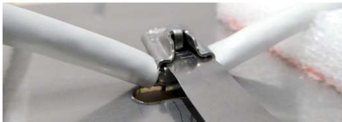
Figure 8.14: Detail of stainless steel tie wrap.
