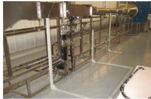
Fig. 14 Wind tunnel testing platform of PFHE fin performance in Hangyang
