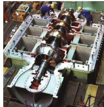
Fig. 5 Assembly of isothermal centrifugal air compressor for 60000 m 3 /h ASU by Shaangu (Ye, 2012)
