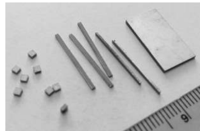
Fig. 4. Piezoceramic plates used to build ultrasonic arrays.
