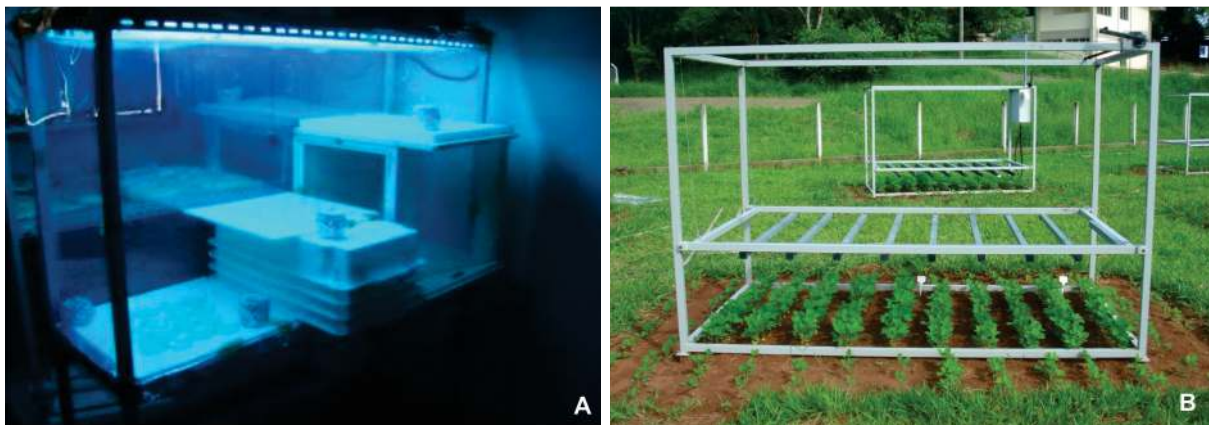
FIGURE 6 - A. Laboratory and B. field facilities to study the effects of increased UV-B radiation on plant diseases and biological control agents (Jaguariúna SP, Brazil).
