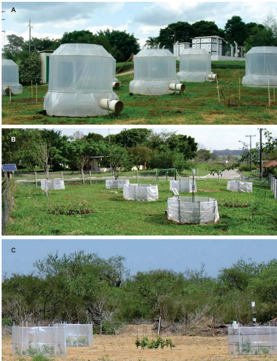
FIGURE 4 - Open-top chambers for studying the impacts of increased air CO 2 concentration (A-B. Jaguariúna SP, Brazil; and C. in Petrolina, PE, Brazil).
