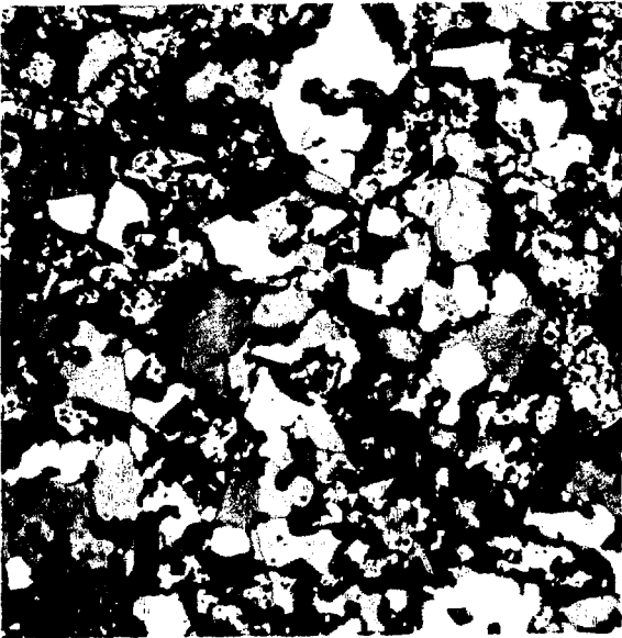
Fig. 4. Photomicrograph of 60% dense extruded ZrC (150X).
