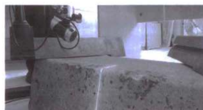
Photo 1. Scanning the surface of reinforced concrete sleeper
