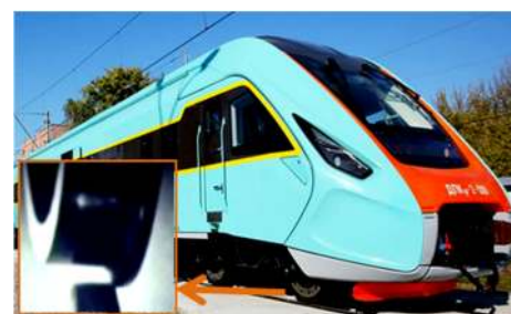
Fig. 1. The wheel rolling onto the head of the rail.
