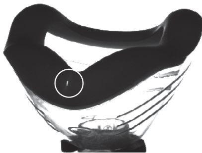
Fig. 8. The defect of the anesthetic mask – a hole in the rubber part. The intensity of hole significantly differs from the intensity in the rubber part of the mask.
