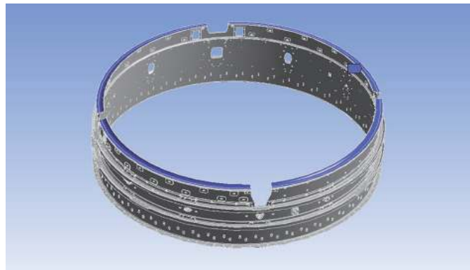
Figure 3-3. Setting of casing boundary conditions
