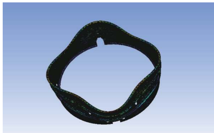
Figure 3-5. Main vibration mode of the casing
