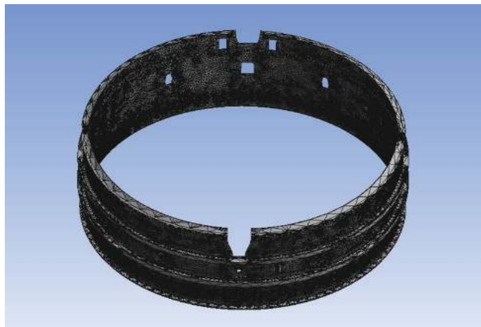
Figure 3-2. Mesh division of the casing
