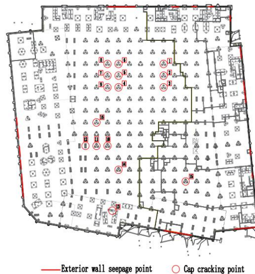
Figure 3. Schematic diagram of water seepage areas and cracking areas
