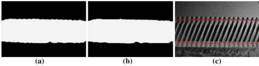
Fig. 6 Segmentation of wheel imprint. a Original classification, b morphological treatment and c segmentation results
