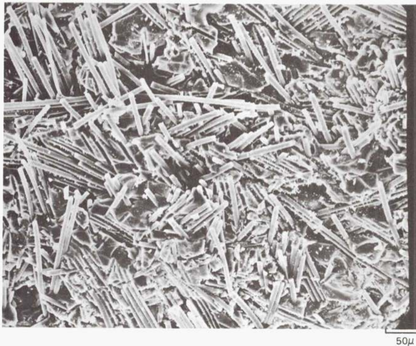
Fig. 35 Fracture Surface of Celion 6000 Paper/7740 Tensile Specimen GC 594-14
