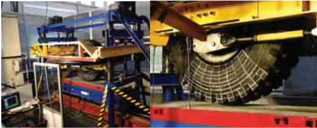
Fig. 4. Laboratory facility for surveys of heavy vehicles tyres
