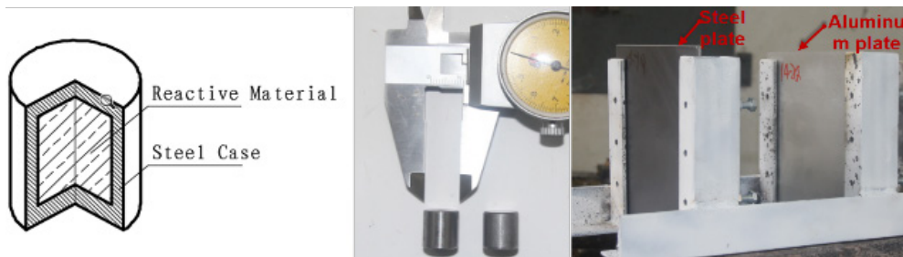
Figure 1: The reactive fragments and double-layer spacing targets
