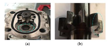
Figure 6. Wear and tear of gear pump: (a) side plate wear; (b) end-face wear of driving gear.
