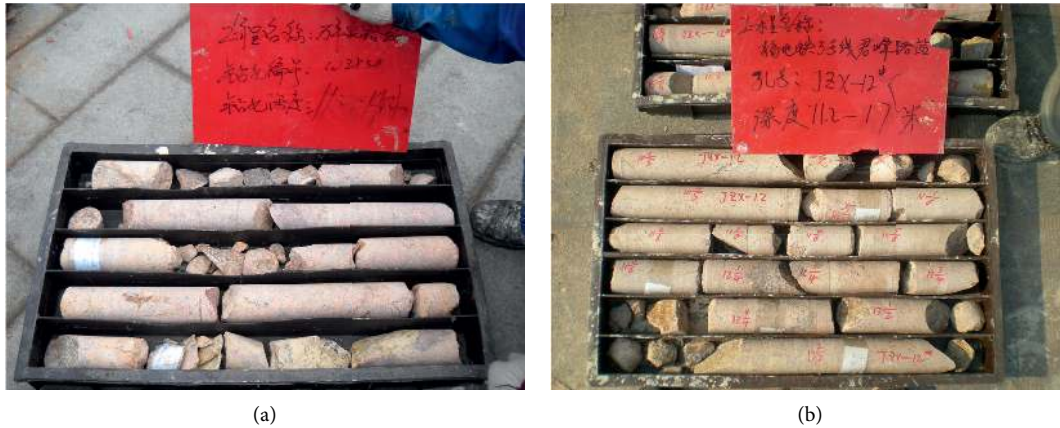
FIGURE 2: Rock drilling sampling diagram. (a) Wannianquan Road Station (b) Junfeng Road Station.
