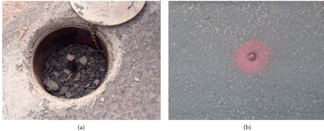
FIGURE 3: Surface settlement monitoring points. (a) Spike. (b) Monitoring stations.
