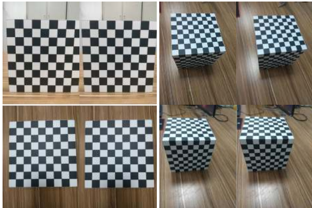
FIGURE 4. Checkerboard images for binocular camera calibration.
