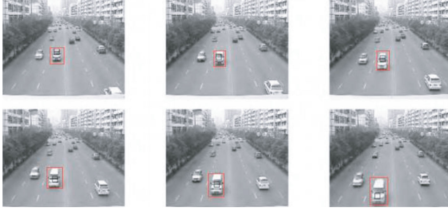
FIGURE 5: Tracking experiment results: tracking effect of white cars. In order to verify the accuracy of the algorithm, the experiment selected a PC configured with Intel core i5 2 GB memory.
