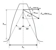
Figure 1. Force on the gear tooth at a boundary point.
