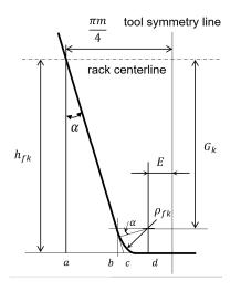
Figure 5. Basic tooth profile of a rack tool.
