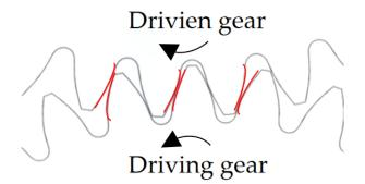
Figure 4. Three-tooth meshing state.
