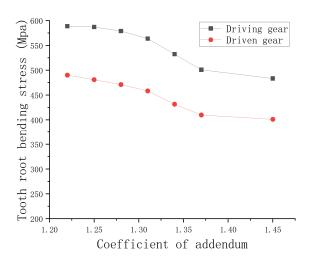
Figure 18. The coefficient of the addendum and tooth root bending stress.
