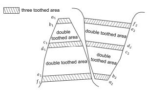
Figure 6. Meshing area of a high-tooth gear pair.
