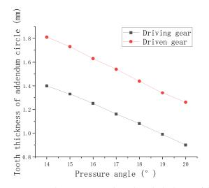
Figure 20. The pressure angle and tooth thickness of the addendum circle.
