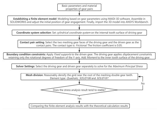
Figure 8. Analysis method flowchart based on FEA.
