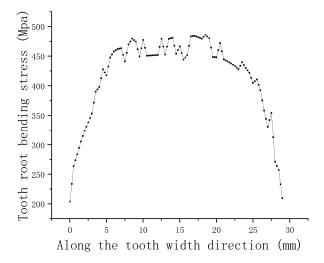
Figure 15. Tooth bending stress distribution.
