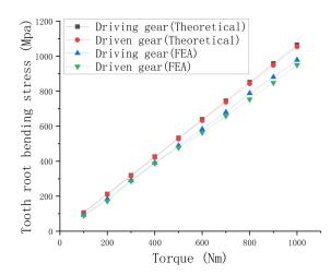
Figure 16. Comparison between theoretical calculation and FEA.
