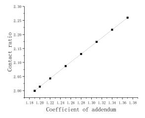
Figure 17. Coefficient of the addendum and contact ratio.
