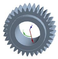
Figure 10. Cylindrical coordinate system.
