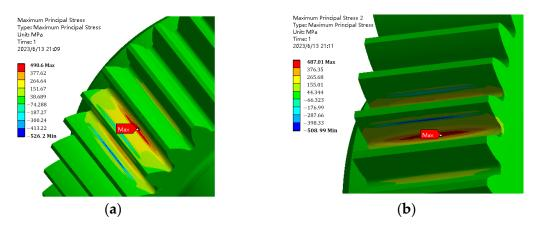
Figure 14. Stress distribution cloud diagram. (a) Driving gear. (b) Driven gear.
