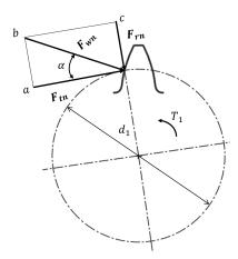
Figure 2. Stress analysis of the high-tooth gear.
