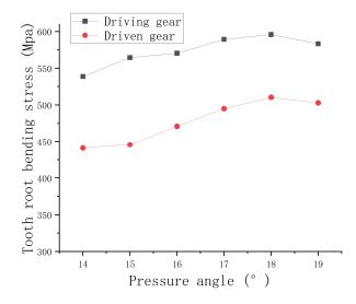
Figure 21. The pressure angle and tooth root bending stress.
