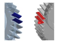
Figure 12. Contact surface of the high-tooth gear pair.
