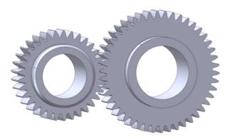
Figure 9. High-tooth gear pair model.
