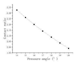
Figure 19. Pressure angle and contact ratio.
