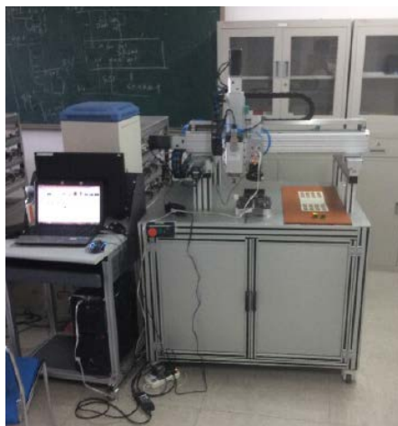
Figure 2. Workpiece sorting system based on machine vision hardware platform.
