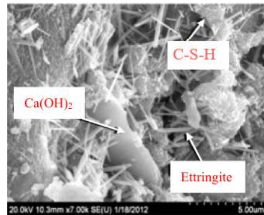
(a) ITZ in old cementitious materials
