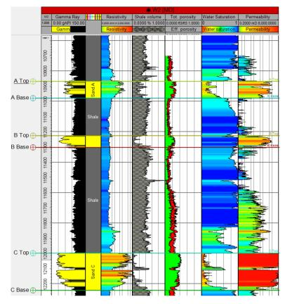
Fig. 5. Petrophysical logs for three reservoir intervals in W2 well
