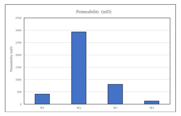
Fig. 10. A plot of permeability for reservoir C sand across all wells
