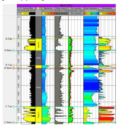
Fig. 6. Petrophysical logs for three reservoir intervals in W3 well
