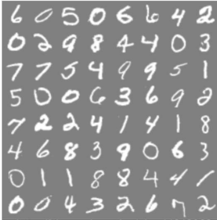
FIGURE 3.3: Sample of handwritten digits from the MNIST database. Each digit image is a matrix of 28 \times 28 pixels with 256 gray-scale levels. Image credit: blog.csdn.net/weixin_44613063 .
