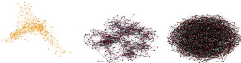
FIGURE 2.10: Comparison of network graphs. Left – C. Elegans biological neural network (277 neurons) [60]. Middle – nanowire network (300 nanowires). Right – random network (300 nodes) [63].
