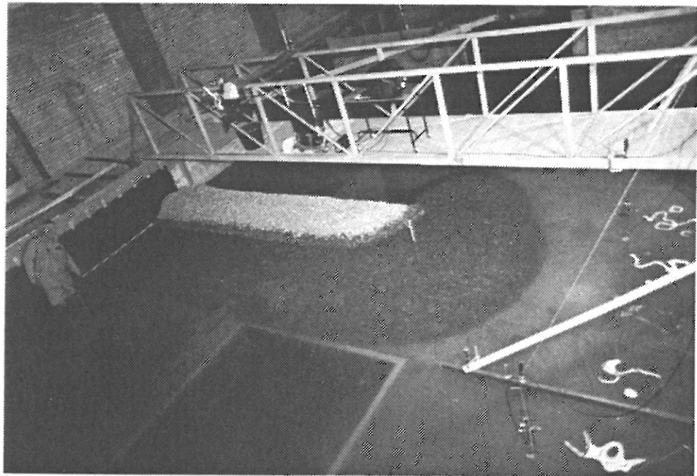
Fig. 11. Photo of the roundhead after exposure to 3000 waves characterized by H_s = 0.15 m and T_p = 2.5 s.
