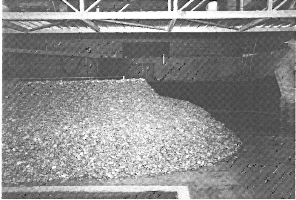
Fig. 10. Photo of roundhead after exposure to 3000 waves characterized by H_s = 0.10 m and T_p = 2.0 s.
