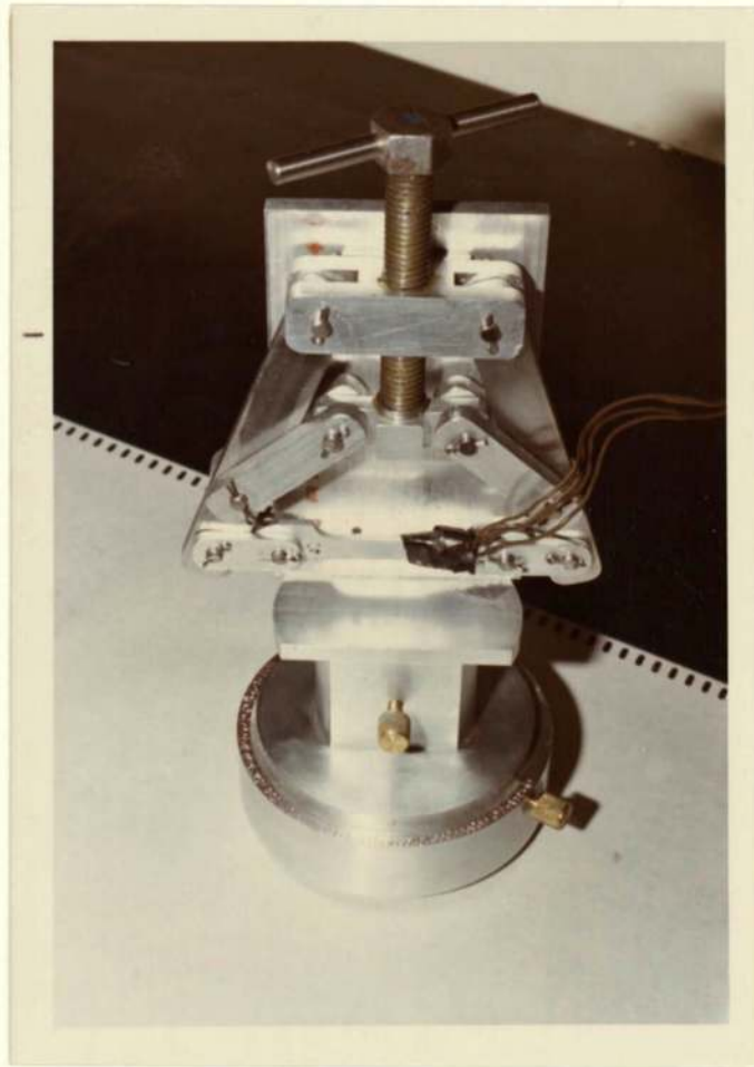
Figure 14. Uniaxial Straining Jig for X-ray Diffraction Stress Measurement Mounted on Specimen Stage, Aluminum Specimen Installed in Place
