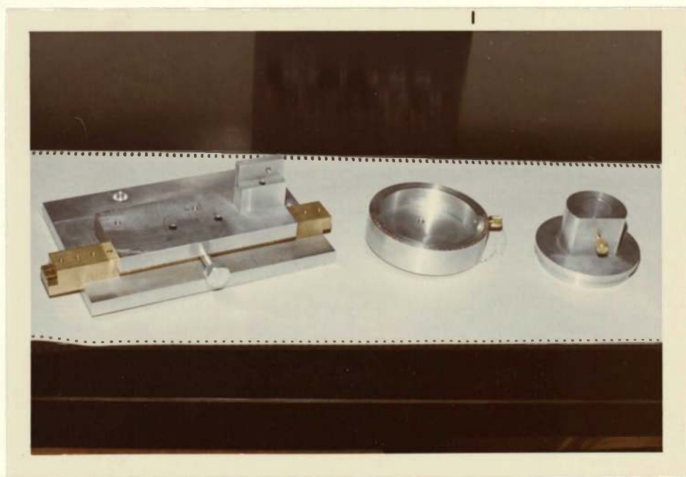
Figure 13. Radially-adjustable Detector Support and Residual-stress Specimen Stage (Two Parts)
