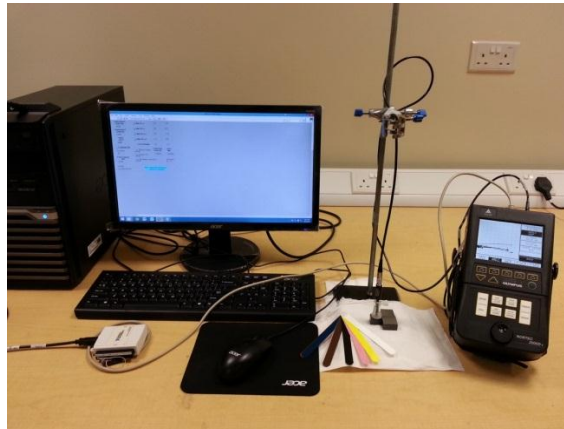
Figure 1. Typical Eddy Current Experimental Set-up for Low Frequency.
