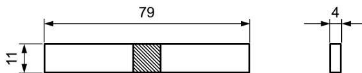
Figure 2: Specimen geometry with peened area (hatched)
