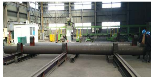
Fig. 3 Specimen after longitudinal butt welding
