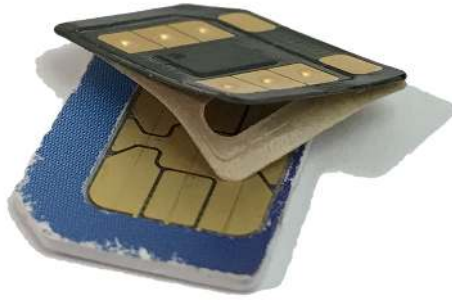
Figure 6.1: An overlay SIM (top) and a regular SIM (bottom). The top part of the overlay SIM can be peeled off and stuck on top of a regular SIM
