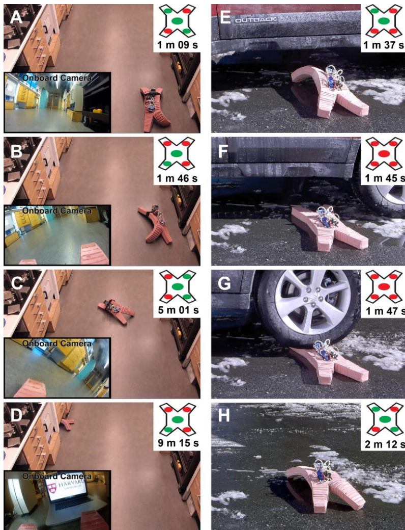
Figure 3. Untethered operation of quadrupedal soft robot. A-D) Untethered soft robot conducting indoor surveillance with onboard camera view overlaid. The robot starts moving forward with a straight ambulatory gait (A). The robot switches to a turning gait to explore a passageway on the left (B, C). The robot uses its onboard camera to image a hidden laptop (D). Green dots on the figures in the upper-right corner of each frame indicate which PNs are currently actuated (pressurized), red dots indicate unactuated PNs. E-H) Untethered soft robot operating outdoors before and after being run over by a car (E). The robot depressurizes its actuators in preparation for impact (F). The car running over the elastomeric legs of the soft robot (G). The soft robot actuating and standing up after being run over by the car (H).
