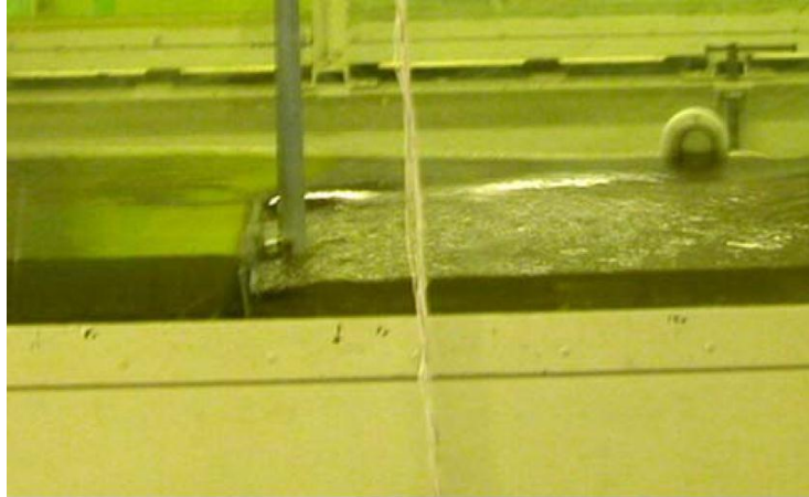
Figure A.2: Submerged plate in flume, from Azinfar 2010.
