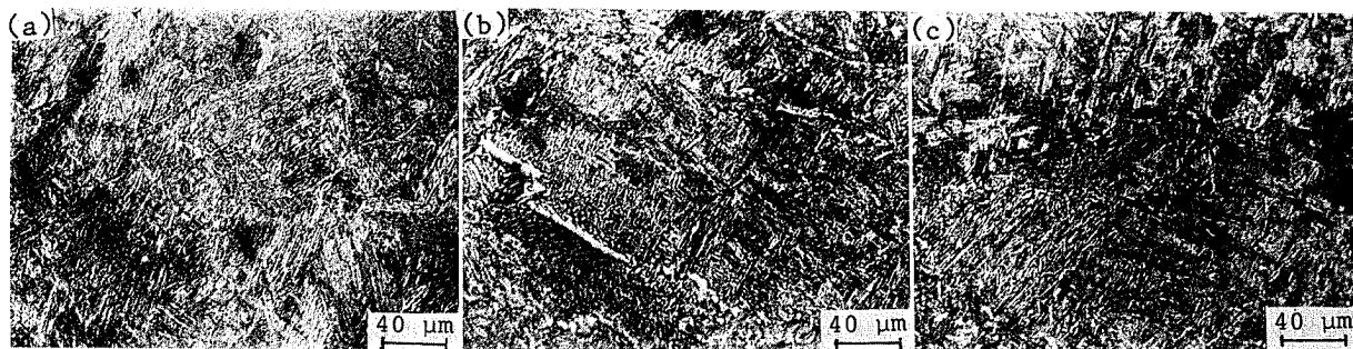
Fig. 9. Influence of effective current on the microstructure of weld nugget, (a) 6 kA; (b) 6.8 kA; (c) 7.4 kA.
