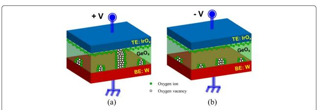
Figure 8 Formation (a) and oxidation (b) of  $Ge/GeO_x$  nanofilaments under SET and RESET operations.  $Ge/GeO_x$  nanowires can be formed under SET and it is dissolved under RESET operations.
