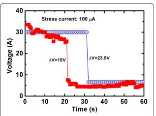
Figure 10 Evolution of voltage shift under constant current stress on the MIM structure. The voltage shift is caused by the filament or NW formation in the  $GeO_x$  film.
