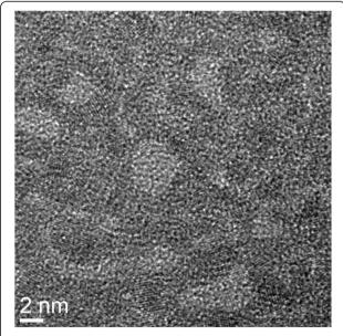
**Figure 6 Plan-view TEM image of an IrO**<sub>x</sub> **layer.** With a typical thickness of approximately 3 nm on the  $SiO_2/Si$  substrate. The  $IrO_x$  metal is black and  $SiO_2$  is white. The  $IrO_x$  metal layer contains pores that oxygen can readily migrate through.
