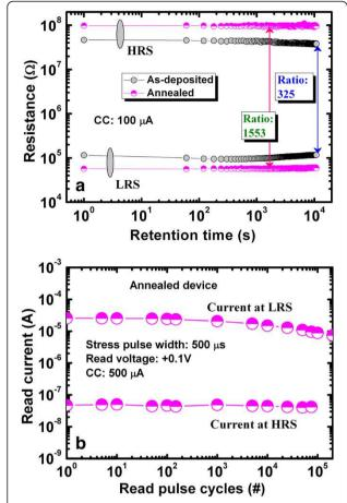
**Figure 9 Data retention characteristics and good pulse read endurance.** (a) Data retention characteristics of the  $IrO_x/GeO_x/W$  devices. The resistance ratio is larger for the PMA devices than that of the as-deposited one after  $10^4$  s. (b) Good pulse read endurance of  $>10^5$  cycles is obtained for the PMA devices.
