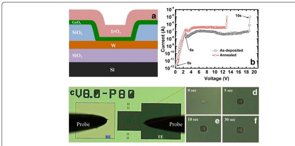
**Figure 5 IrO**<sub>x</sub>/GeO<sub>x</sub>/W MIM structure, typical *I-V* characteristics, and migration of oxygen ions. (a) Schematic diagram of the IrO<sub>x</sub>/GeO<sub>x</sub>/W MIM structure. (b) Typical *I-V* characteristics of as-deposited and PMA devices. (c to f) The migration of oxygen ions during application of a formation voltage, as shown in (b).
