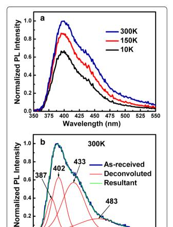
Figure 3 PL and deconvoluted spectra. PL spectra of the Ge/GeO<sub>x</sub> NWs (a) measured at temperatures of 10 to 300 K and (b) deconvoluted spectra at 300 K.
