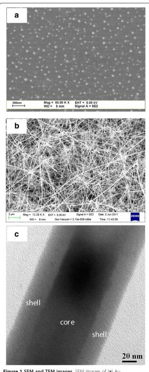
Figure 1 SEM and TEM images. SEM images of (a) Au nanoparticles and (b) Ge NWs on Si substrates. (c) TEM image of core-shell Ge/GeO<sub>x</sub> NWs.
