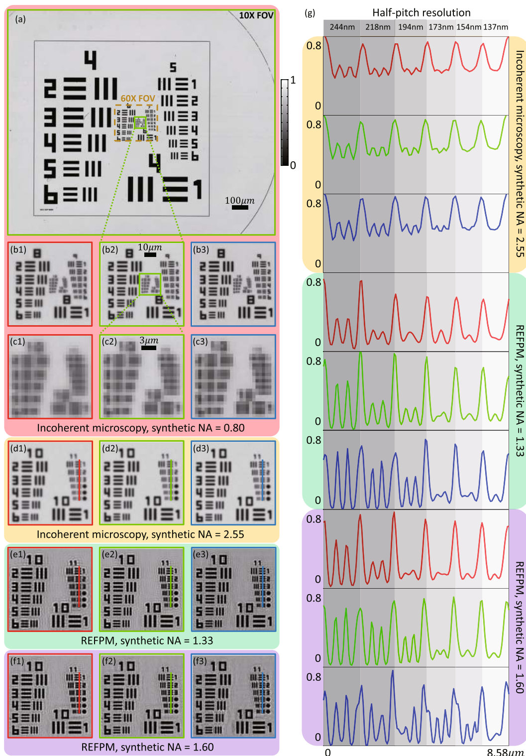
Figure 1. Imaging and recovery results of conventional bright-field microscopy and REFPM systems for the same USAF resolution target. (a) The full FOV of the incoherent microscopy image using a 10 \times 0.4 NA objective lens with 0.4 NA illumination. (b,c) Enlarged sub-regions of Fig. 1(a) in R/G/B channels. (d) High-resolution incoherent microscopy results using a 60 \times 1.35 NA objective lens with 1.2 NA illumination in three channels. (e,f) REFPM recovery results obtained by employing a 10 \times 0.4 NA objective lens with 0.93 NA and 1.2 NA illumination in R/G/B channels. (g) Line-scan profiles from the selected position of targets in Fig. 1(d1–f3).
