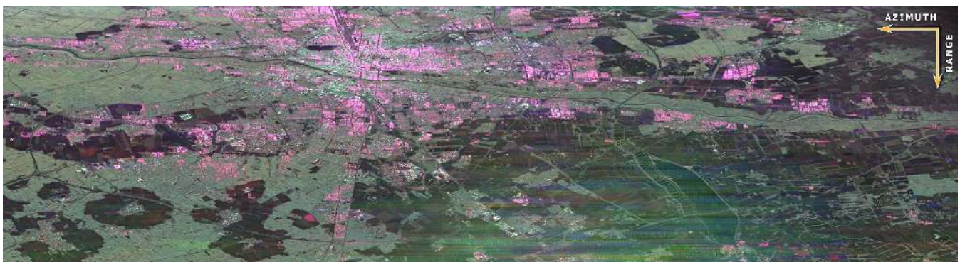
Fig. 14. SLC SAR image of the test site in Munich, Germany, 2015 (near range on top). The colors correspond to the channels HH (red), VV (blue) and HV (green).
